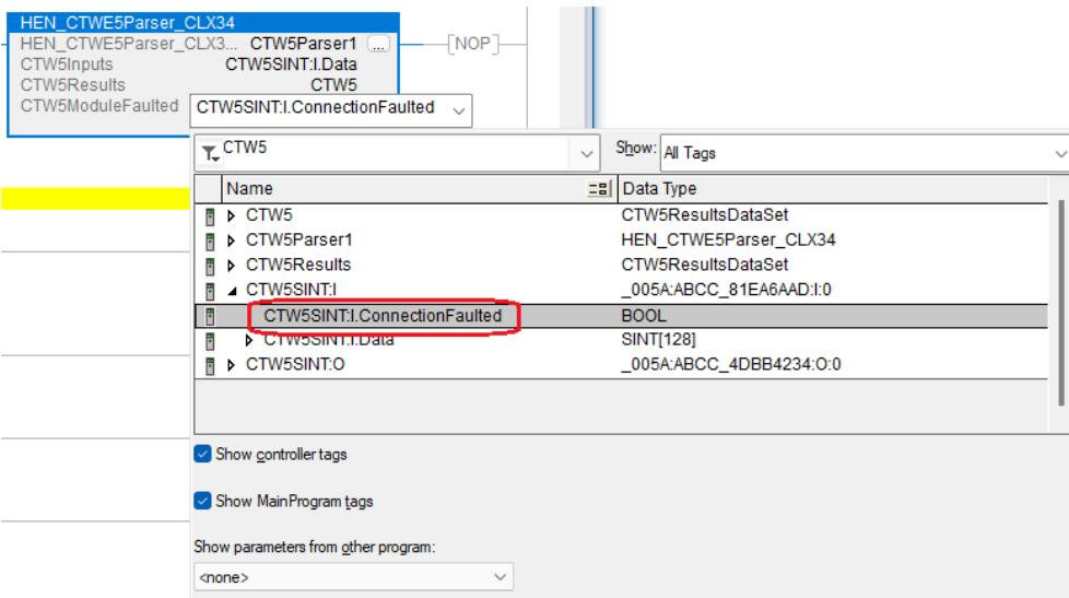
Parses the INT[64] input byte array from a Heraeus CTW5 whose EIP output communication is configured to use the Telegram #10. The received data is parsed into 1 userdefined CTW5ResultsDataSet structure.
